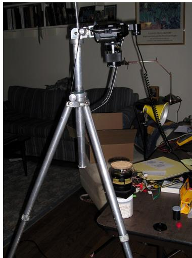
Figure 6: The camera and shaker setup for taking pictures of the pattern. The SLR is shown, but the video camera was mounted in a similar manner.
